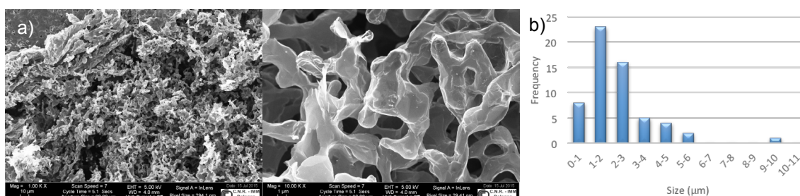
Figure 2. a) SEM images of graphene foams from sintered Ni nanoparticle templates at increasing magnification and b) corresponding pore size distribution
