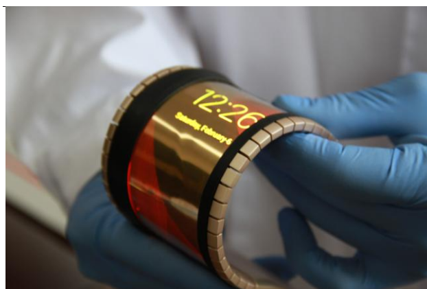
Figure 2: Flexible mobile phones with graphene transparent conductive film
