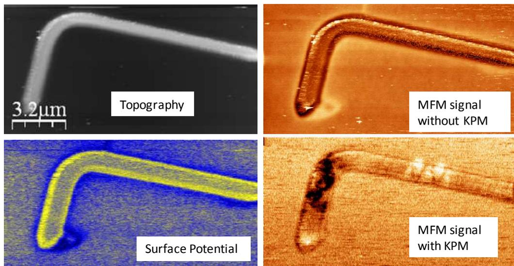
**Figure 1:** (a) Topography and (b) MFM signal (frequency shift) of a cobalt nanostripe without electrostatic compensation. The contrast drastically changes when KPM is used simultaneously: (c) Surface potential image and (d) MFM signal with KPFM.
