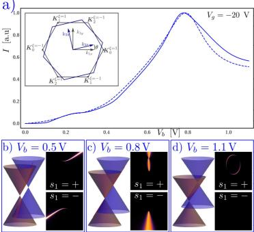
**(a)** The measured (solid curve) and theoretically calculated (dashed curve) tunnelling currents, displaying the resonant peak at a bias voltage of  $V_b$ ≈0.8V.
